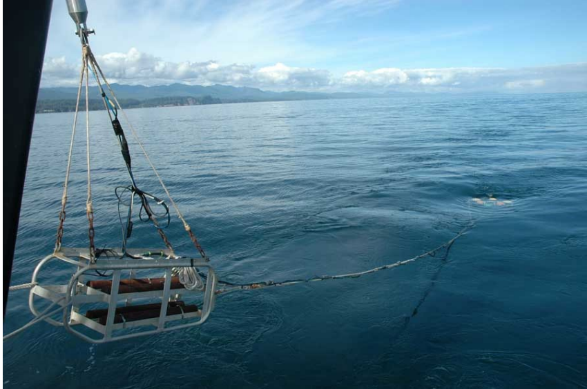
Figure A-28 TACOS video system during deployment
