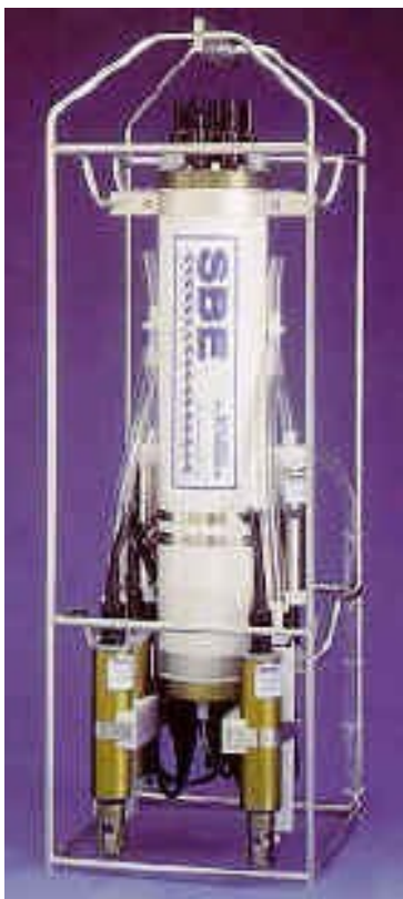
Figure A-22 Sea-Bird 911 and CTD deployment on a sampling rosette with Niskin bottles
