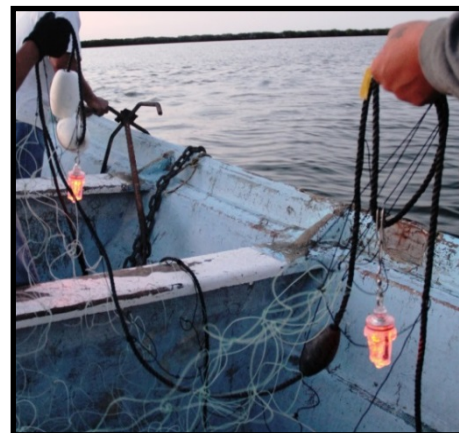
Figure 5.3. LED trials to determine potential reduction of elasmobranch bycatch in gillnets.
