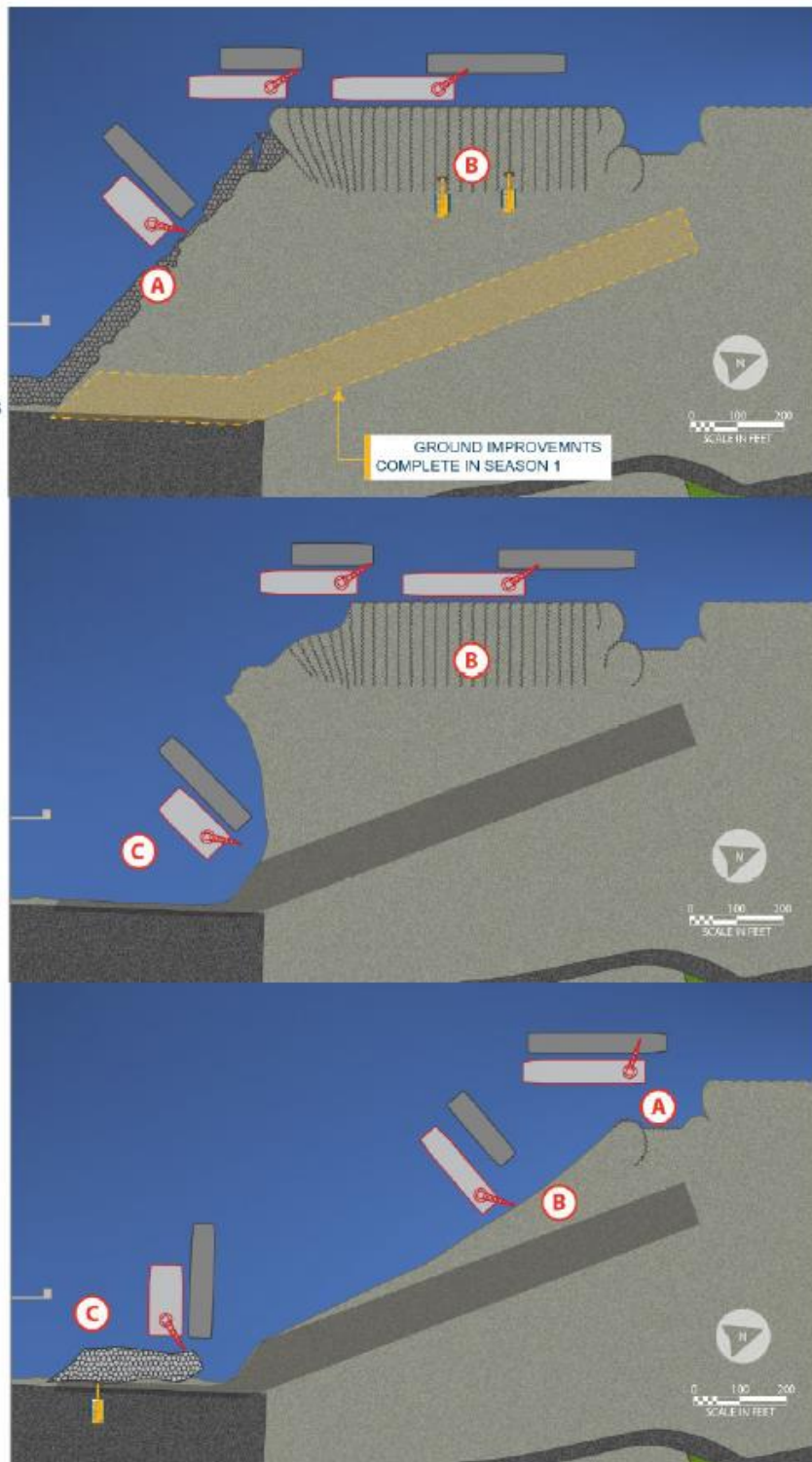
Figure 6. Example of the Contractor's Proposed Demolition Plan
