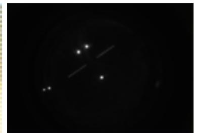
A raw (above) and processed (below) image of a harmful algae array from the ESP. The brightness of the dots is representative of the abundance of the target harmful algal species.
