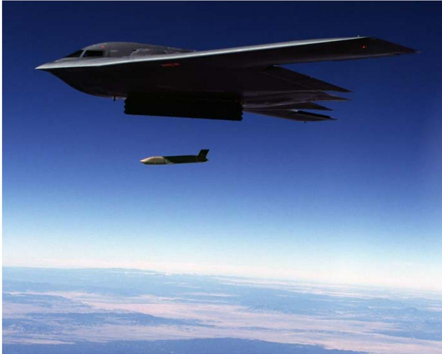
**Figure 1-2. Joint Air-to-Surface Stand-off Missile (JASSM) in Flight**
