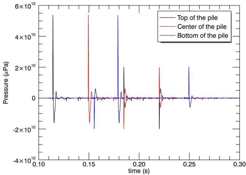
Figure 4. Example of a wavelet at three points (top, center, and bottom) along the pile.
