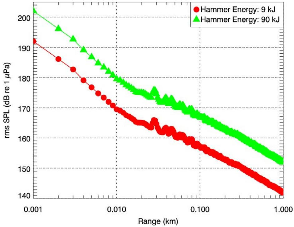
Figure 8. Root-mean-square sound pressure levels (rms SPLs) as a function of range south of the pile driving operations, for the minimum (9 kJ) and maximum (90 kJ) hammer energy.
