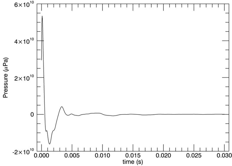
Figure 3. Wavelet derived from the 1/3-octave-band source level spectrum associated with 90 kJ hammer energy (black; Figure 2).
