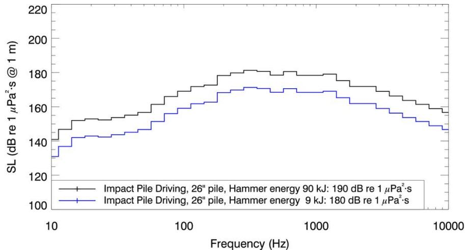
Figure 2. Estimated 1/3-octave-band source level spectra for impact pile driving a 26-inch pipe pile associated with 90 kJ (black) hammer energy and 9 kJ (blue) hammer energy.
