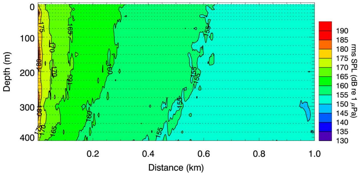
Figure 7. *Maximum Hammer Energy (90 kJ)*: root-mean-square sound pressure levels (rms SPLs) along depth and range south of the pile. Dotted lines represent depths at which received levels were modeled. In this figure, values between modeled depths were linearly interpolated.
