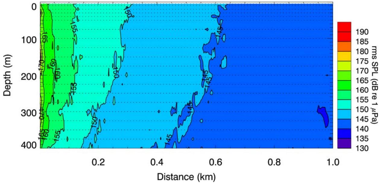
Figure 6. *Minimum Hammer Energy (9 kJ)*: root-mean-square sound pressure levels (rms SPLs) along depth and range south of the pile. Dotted lines represent depths at which received levels were modeled. In this figure, values between modeled depths were linearly interpolated.
