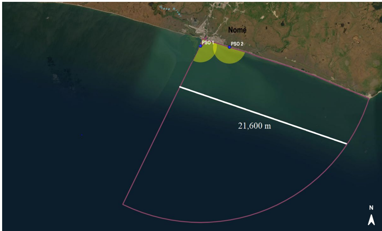
Figure 5. Level B harassment zone for 36” fender (pipe) piles is outlined in purple (zone has a radius of 21,600 m). The yellow shaded area is the area that a PSO can reliably observe marine mammals. Zone location is not fixed; it would change as the causeway is built out.
